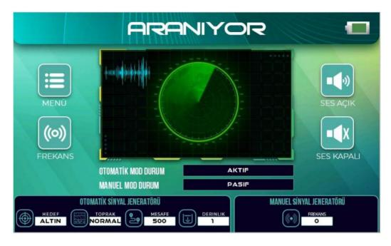
In order to define the frequency values displayed on the previous screen to the device, first the MENU button must be pressed.
