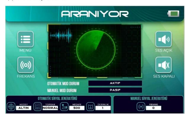
Then, the relevant probes for the Automatic Signal Generator are attached and the connection to the piles previously driven into the ground is completed. The device should remain on for a minimum of 45 minutes and should not be interfered with in this mode. Then the search can be started with the help of a handheld eliminator.
