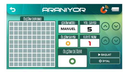
After determining the number of Ways for the area to be shot, it is adjusted with the help of the up and down buttons in Figure 11. Then the Registration number is set to save it in a memory that you know is empty before. After the necessary adjustments are made, the measurement is started by pressing the Start button.
