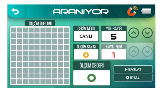
With this mode, it is necessary to press the measurement button for each measurement. Measurements can be displayed on the interface each time the measurement button is pressed.
