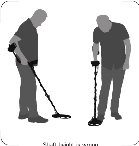
Shaft height is wrong
